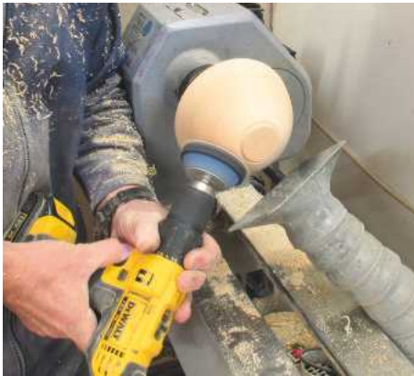
▲ Pic.4 Power sanding is the other option, along with doing it by hand. A drill mounted arbor is held in the 8 o'clock position. Try to get as much of the pad into contact with the bowl surface as possible
